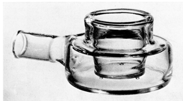
Fig. 1. Culture flask for cinematography.
